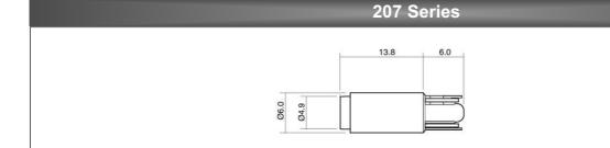
Dimensions in mm (Typical) Not to scale Green dot on base indicates anode +ve. Colour dot on product denotes LED colour
